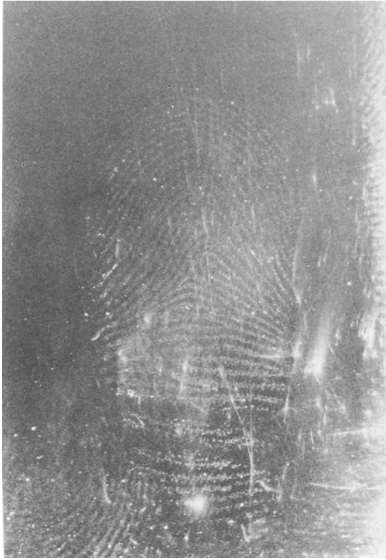
FIG. 7—Weak latent print on glass developed by all-lines blue-green Ar laser excitation. The print was visible to the eye under the Ar laser.
