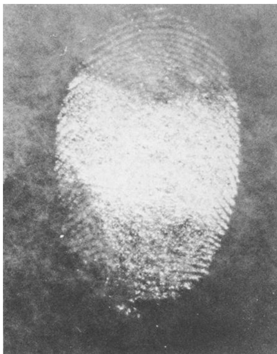
FIG. 3—Latent print dusted with rhodamine 6G-blended magnetic powder and developed by frequency-doubled Nd:YAG laser.
