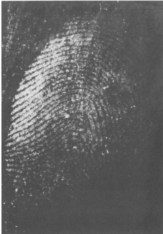
FIG. 1—Latent print on paper developed by frequency-doubled Nd:YAG laser (inherent fingerprint fluorescence).
